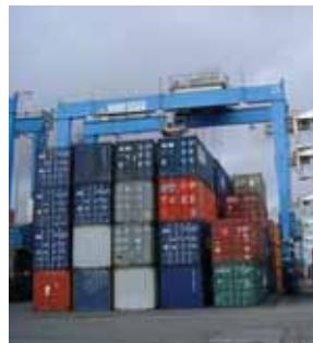
The Maxview vision system, added to the basic Maxspeed control system and CraneDirector™ crane automation interface, provides several levels of scalable crane automation from semi-automatic with manual assistance up to fully-automatic, unmanned operation:
