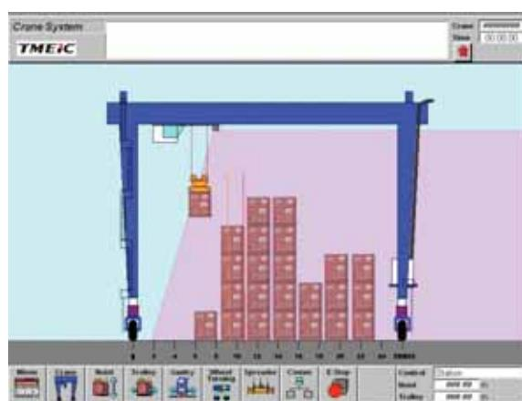
Maxview Smart Move system on an RTG Crane
