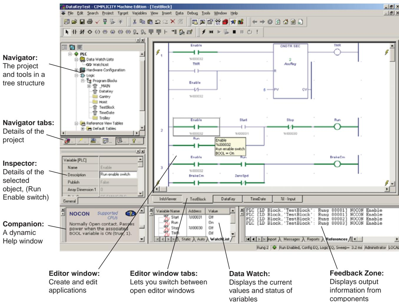
The screen above shows a typical layout of the tools and editors available. The editor window shows a ladder logic diagram with real-time data and power flow displayed in green. In addition to the windows shown above, two other windows can be added:
